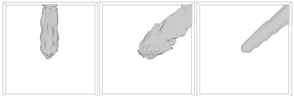
Figure 5: Comparison of the dispersion in different directions and with the improved approximation (iso-area for concentration 1 OU/m<sup>3</sup>; central point source 5 MOU/h at a height of 8 m; wind speed 2 m/s)
