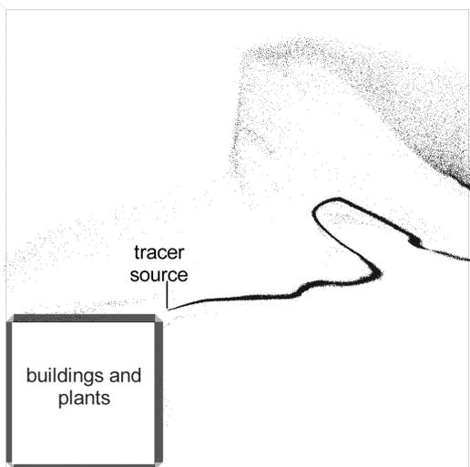
Figure 7: Meandering dispersion plume of a point source, calculated with the NaSt3D model and the Lagrange dispersion approach
