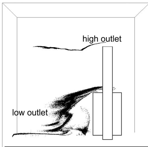
Figure 6: Comparison of the dispersion of substances behind a low and a high emission source, calculated with NaSt3D and the Lagrange particle model
