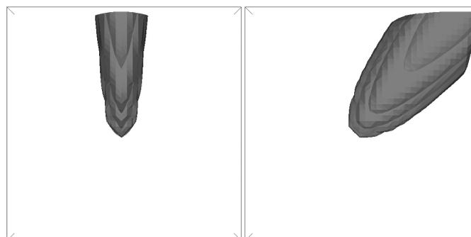
Figure 3: Numerical diffusion caused by a flow at 45° to the grid direction, as compared with a flow parallel to the axis, calculated with MISKAM (iso-area for concentration 1 OU/m<sup>3</sup>, odour source: central area source 11 MOU/h at a height of 8 m; wind speed 1 m/s)
