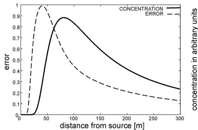
Figure 2: Development of the concentration with the relative error of the Gauss model, calculated using the dispersion class III/1 at a height of 2 m as an example
