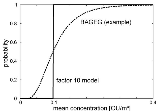
Figure 1: Probability of the odour threshold being exceeded by 10% according to the factor 10 model (leap at 0.1 OU) and the BAGEG model (functional connection)
