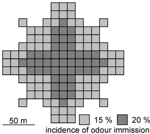
Figure 4: Influence of numerical diffusion on the annual prediction of the odour input of a central point source if wind statistics are symmetrical, calculated with MISKAM and the factor 10 model (wind speed 1 m/s in 36 directions; source see above)
